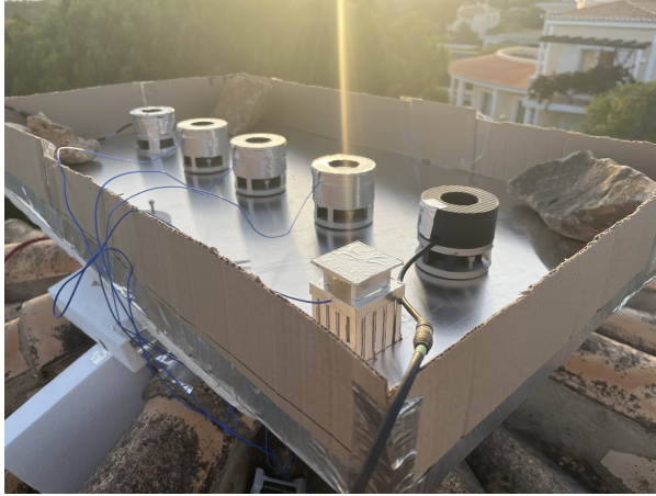
(a) Experimental setup on the roof showing (from background to foreground): pyrometer, apparatuses A, B, and C, and pyranometer. The air temperature sensor housing is visible in the foreground corner.
